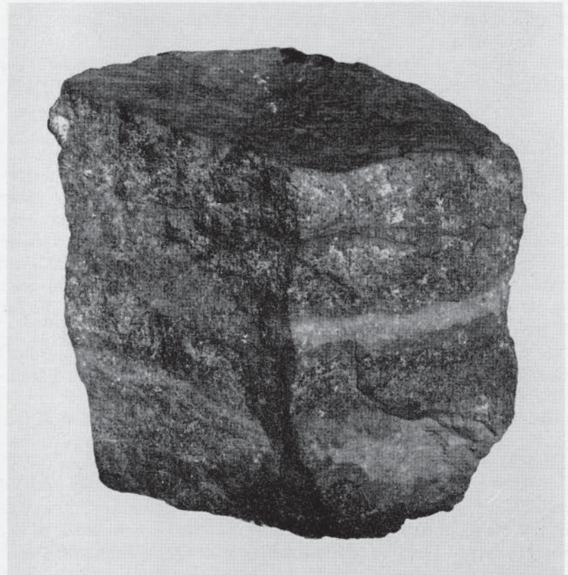
FIGURE 11. Garnet-diopside layers in metamorphosed member 1 of the Secret Canyon shale. Garnet layers, representing original shale beds, are dark and coarse-grained. Diopside layers, representing original limestone beds, are light and fine-grained.
