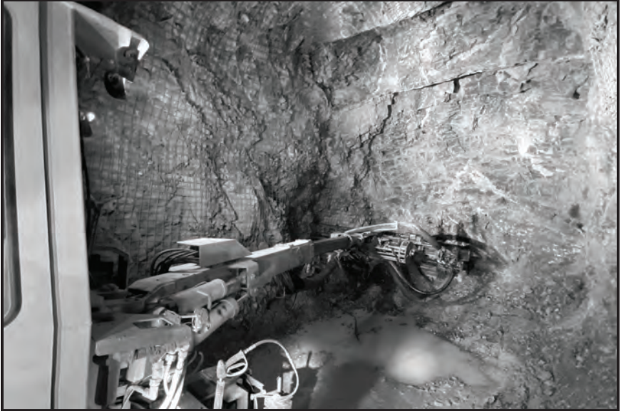
Bolter at Cove underground gold mine, Lander County (i-80 Gold Corp. photo).
