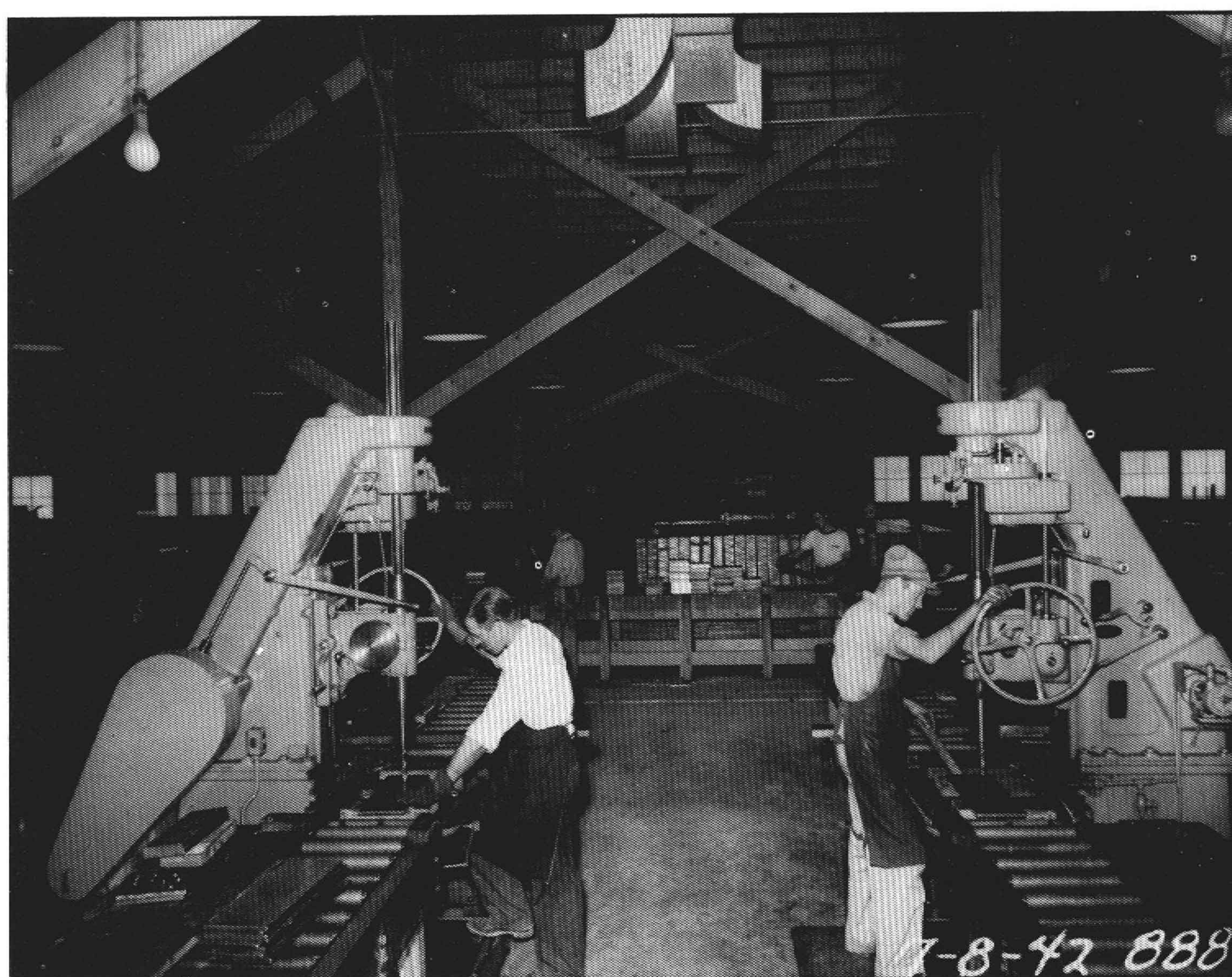
Workers at Basic Magnesium drilling 7/8" holes in busbars, July 8, 1942. (Kunkel Collection, University of Nevada, Las Vegas Library)
