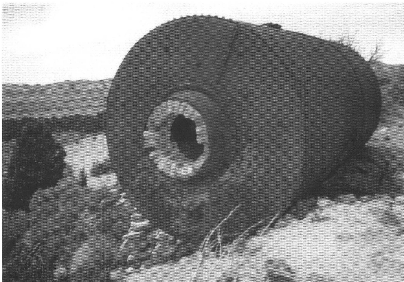
The Bruckner furnace for batch chlorination. Two of the furnaces can be seen on the extreme right in the photo on page 297. (Collection of the Author)
