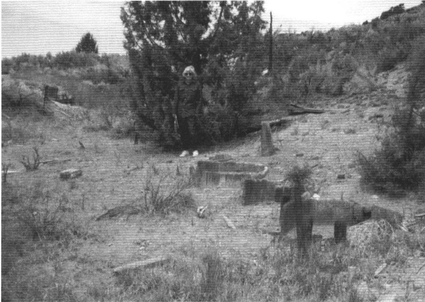
Eleven half-buried wooden barrels in a straight line, probably amalgam settlers. (Collection of the Author)
