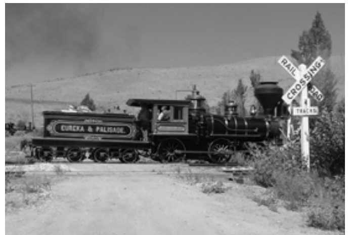
Dan Markoff of Las Vegas brought his Eureka , 36-inch gauge steamer originally from the Eureka & Palisade RR. Still burns wood.
