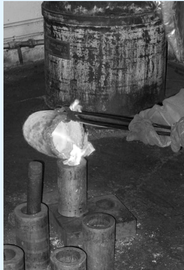
Pouring molten Nevada silver into a metal mold.
