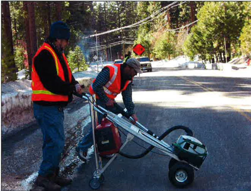
Sampling for sweeper efficiency on Village Blvd.
