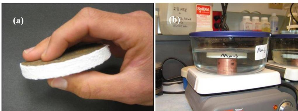
Figure 3. (a) Prepared core wafer section; (b) matrix diffusion reactor on stir plate ready for sampling.
