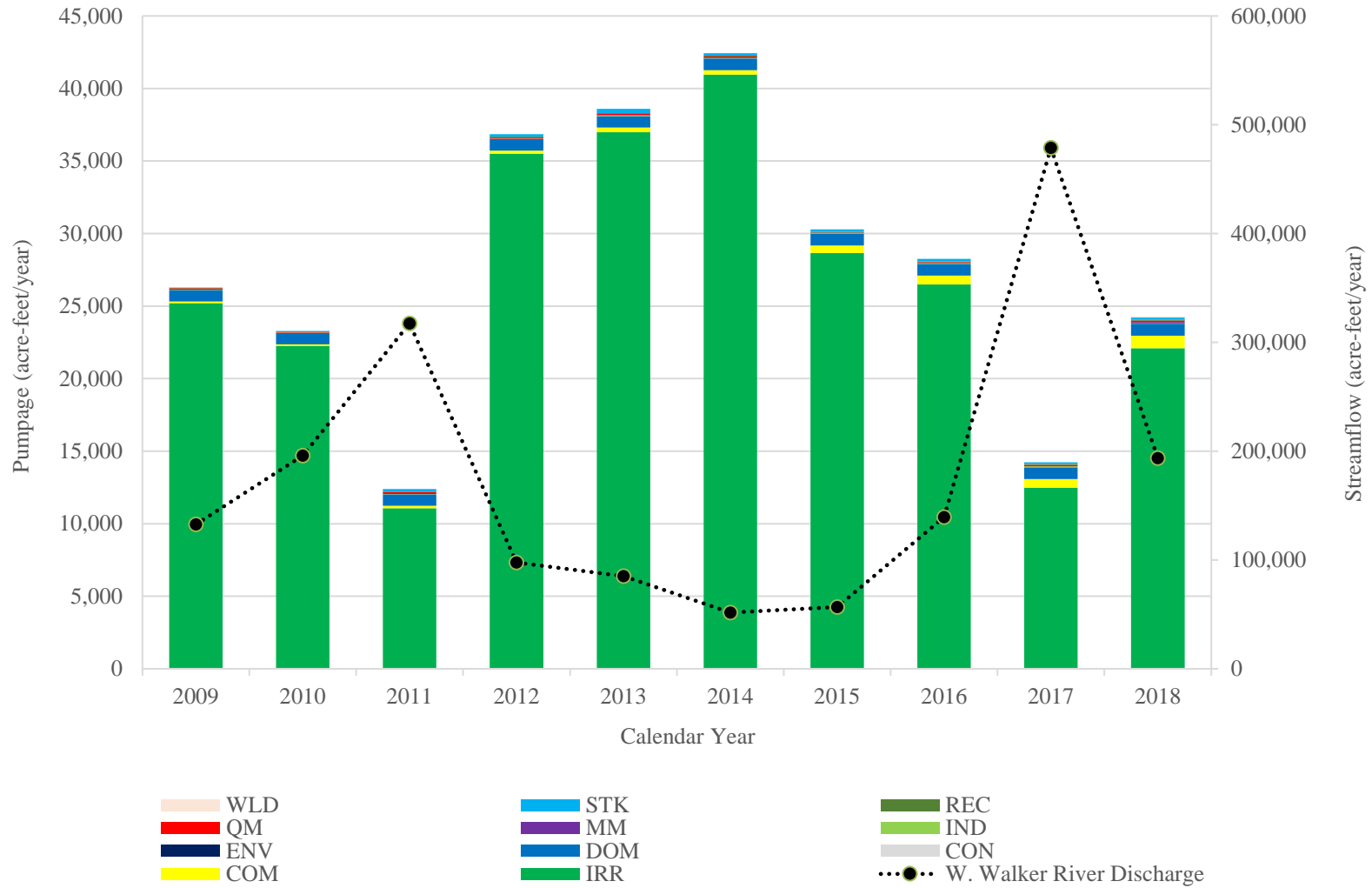
Figure 3. Smith Valley historical pumpage by manner of use as compared with West Walker River streamflow at Hoye Bridge. Note: Prior to 2011, pumpage use monitoring was mostly limited to larger users/wells.
