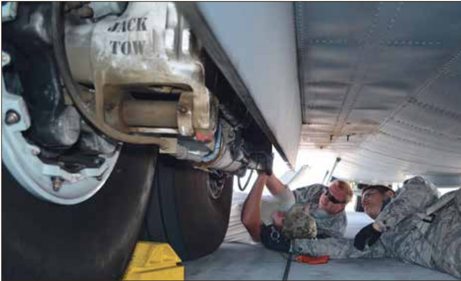
Staff Sgt. Ron Hanselman, Master Sgt. Mike Faulkenberry and Staff Sgt. Tom Kinney of the 152nd Maintenance Squadron's Crash Recovery Team lock the struts on a C-130 in order to simulate repairing an aircraft with flat tires on May 29, 2014.
