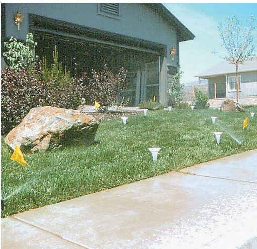
A catch can test is performed as part of a water audit.
