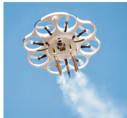
Drone America's DAX8 flies with silver-iodide cloud-seeding flares in northern Nevada.
