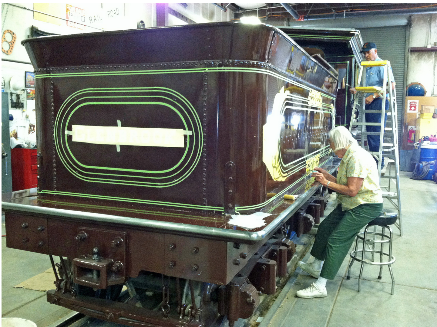
Jim Ingram and his wife, Lorna, apply gold leaf to the Glenbrook's tender and cab on September 29, 2014. Jim has extensive experience painting steam locomotives, including work on the Jupiter and 119 at Golden Spike National Historic Site at Promontory Summit, Utah, and the Central Pacific's Leviathan, which was recreated at the Kloke Locomotive Works of Elgin, Illinois. NSRM Photo.
