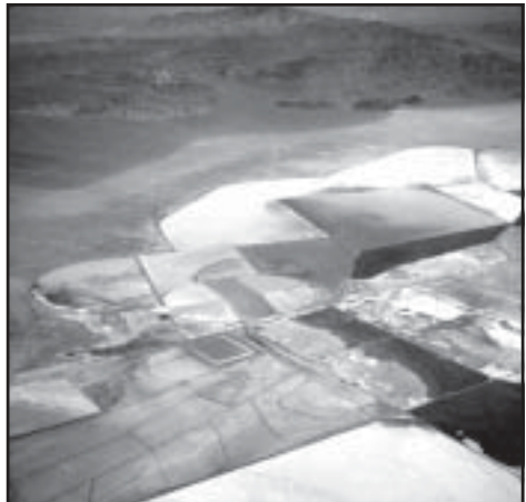
Lithium brine evaporation ponds (NDOM photo)
