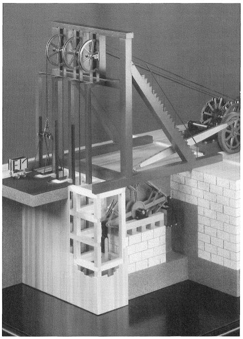
A scale model of the Savage shaft headframe and pump bob. The horizontal pitman rod connects the engine to the pump bob. The wooden pump rod is hanging vertically in the shaft. (*Author's collection*)
