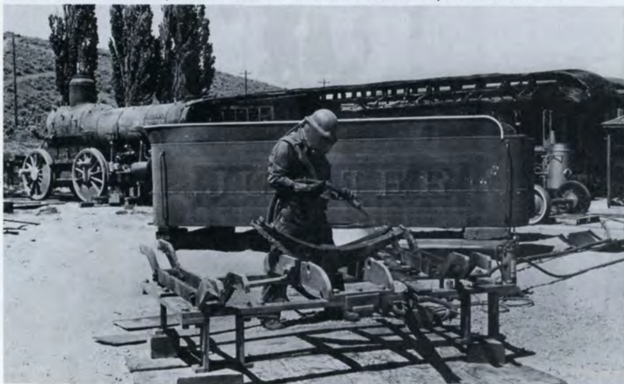
Back from Utah, the old Inyo engine and tender get sandblasted by craftsman Kim Horn.
