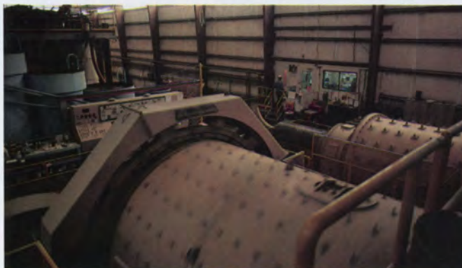
To make invisible gold appear, the Pinson Mine northeast of Winnemucca relies on science and power. Above left, a technician tests gold by melting it in a porcelain crucible in the assay lab. Within the mill, ball crushers turn rock into powder. At right, giant machines carve a profit from raw ore.
