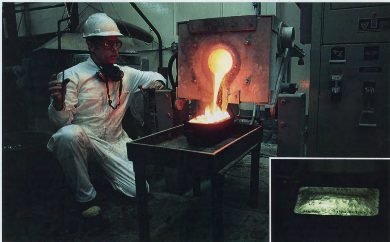
Pinson Mine refiner Mike McDermott watches molten gold fill a crucible. The slag spills over the top, while the gold sinks to the bottom. The outfit pours a 75-pound bar (inset) about once a week—nearly 300 to date. The bars assay out at 98 percent gold and 2 percent silver.
